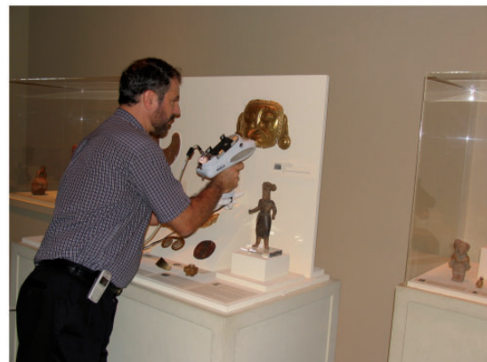
Figure 11. Nondestructive analysis of “gold” mask from Colombia, in Orlando Museum of Art display case.
