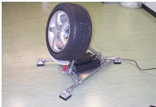
Fig. 45. Tyre Pressure Monitoring System incorporating the amorphous alloy wireless, battery-free sensor (courtesy A. Bowles [339]).
