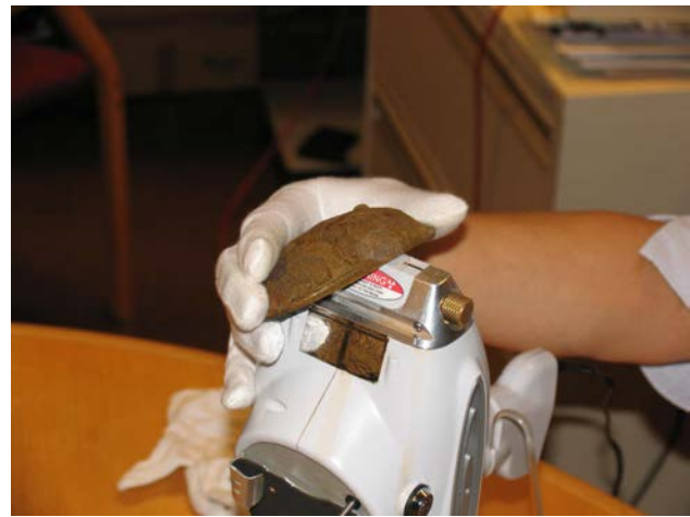
Figure 36.4. Viking Age cruciform brooch, Stavanger Museum, Norway. Analysis of inner edge by pXRF
