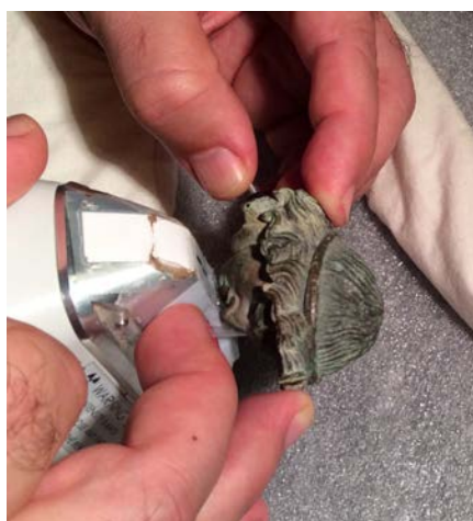
Figure 36.2. Portable X-ray fluorescence analysis of a small “bronze” head at Emory University
